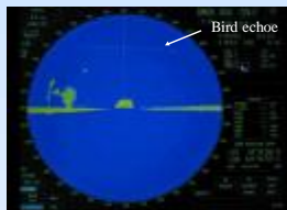
Radars screen with the echo of a bird passing Nysted offshore windfarm.
