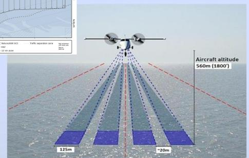
Figure 2: Configuration and orientation of the four video cameras for digital aerial surveys.
