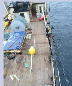
Fig. 1. WDS buoy with C-POD on the deck of research vessel.
