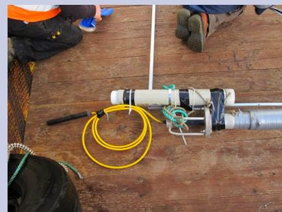
Fig. 2. WDS hydrophone (yellow cable) with C-POD.
